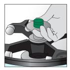
Push center button to remove rotor
